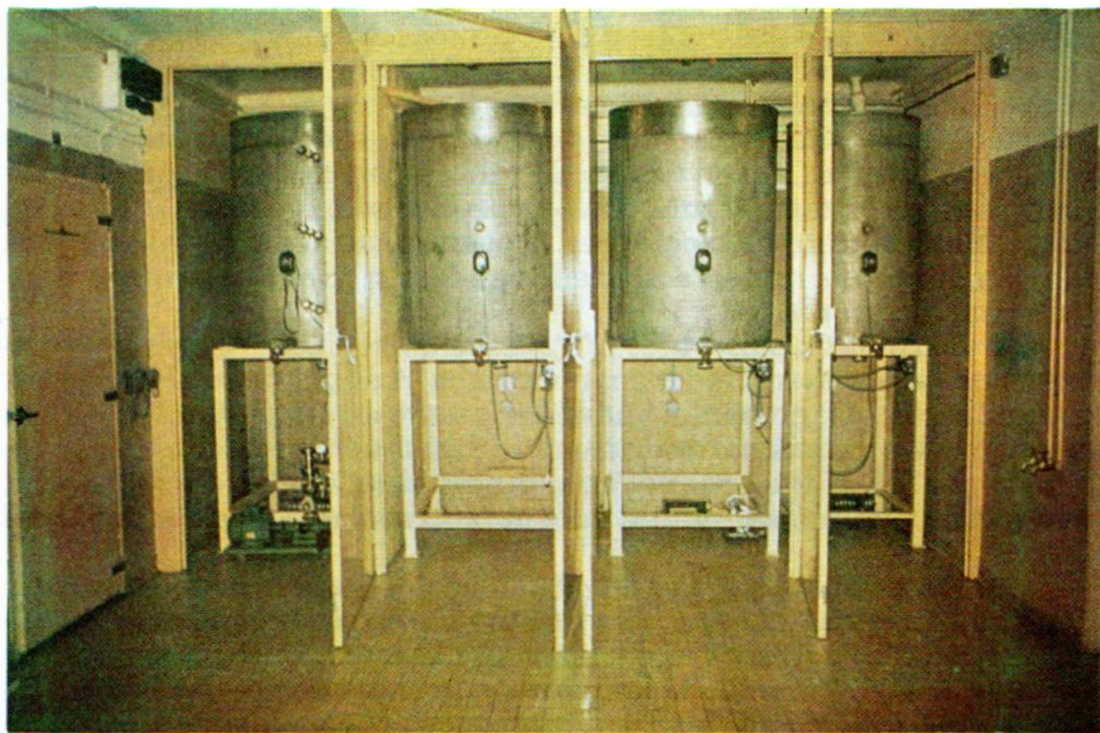
V. Fig. 7 — Decantation basins used for honey. These receptacles are made of stainless steel. Aluminium can also be used, as well as any alloy or plastic material with a food label. (Photo M. Gonnet)
